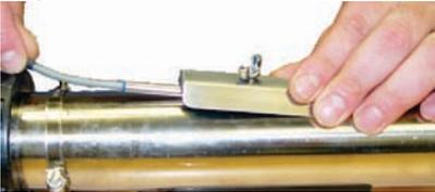
Insert the 1/4 dia. sensor probe under the sensor cover attached to the heater and tighten the wing-nut to secure.
