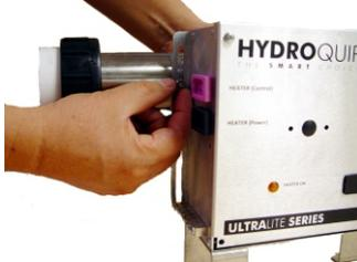
Align the other studded clamp and attach to the other slide bracket. Now determine the proper alignment for the heater and tighten the nuts and clamps.
