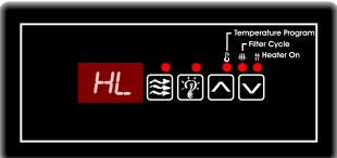
If the water temperature exceeds 112°F at the systems temperature sensor (located in a plumbing dry-well or in wet-well in the spa) the system will shut off the heater and all other outputs will be disabled (pump) until the water temperature drops below 110°F.
