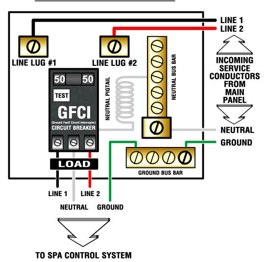
LOAD NEUTRAL <u>MUST</u> BE CONNECTED DIRECTLY TO GFCI AS SHOWN
