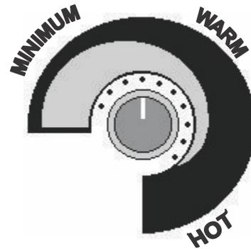
The graduations on the scale around the thermostat are intended for reference points only. They do not reflect the actual temperature of the water. Make small adjustments until the desired temperature is achieved. Allow several hours between adjustments for the temperature to stabilize. Use an accurate thermometer to monitor the water temperature.
