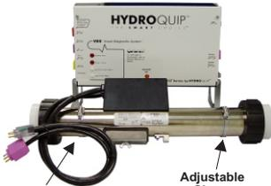
When the adjustable clamps are mounted to the heater, adjust the stud locations to align with the slide brackets on one end. Do not tighten nuts yet.
