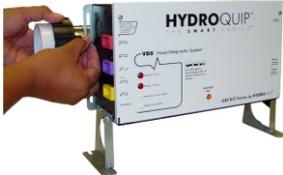
Align the other studded clamp and attach to the other slide bracket. Now determine the proper alignment for the heater and tighten the nuts and clamps
