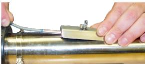
Insert the sensor probe(s) under the sensor cover attached to the heater and tighten the wing-nut to secure.
