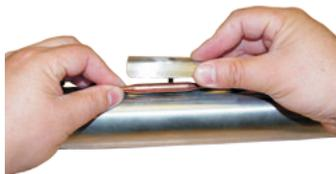
Insert the sensor probe(s) under the sensor cover attached to the heater and tighten the wing-nut to secure.
