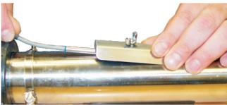
Insert the sensor probe(s) under the sensor cover attached to the heater and tighten the wing-nut to secure.
