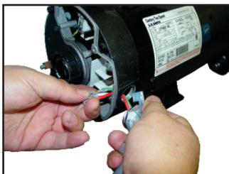
3) Route the power wires through the conduit hole and pull toward you to allow for the cord assy to be rotated for tightening.
