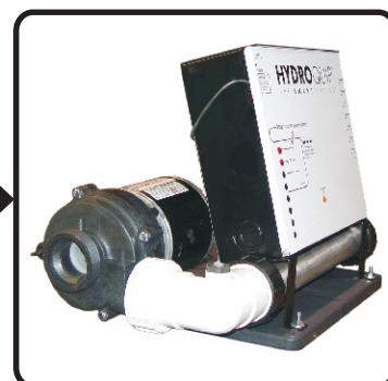
Fig. 12 - Tighten the pump to heater header making sure gasket and O'rings are present. Unit is now assembled and ready to install.
