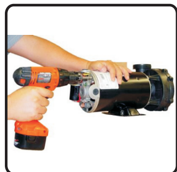
Fig. 1 - Loosen the four(4) retaining thru bolts
