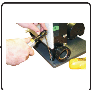
Fig. 11 - Secure control using the mounting hardware provided
